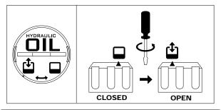
Use a screwdriver to rotate the centre part of the breather cap. The triangle indicator on the cap should be aligned with the image on the top of the cap to show "CLOSED" or "OPEN".
